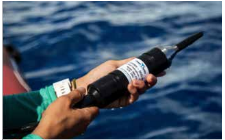
A researcher deploying the icListen Hydrophone. Photo: Ocean Sonics
