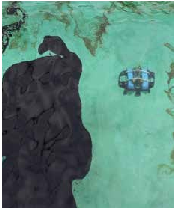
Oil spill tracking with an ROV at the Ohmsett tank in New Jersey
