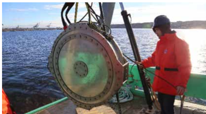
These are C-Bass transducers. They can make very-low-frequency sounds and can even play rock music into the water. Photos courtesy of GeoSpectrum Technologies Inc.
