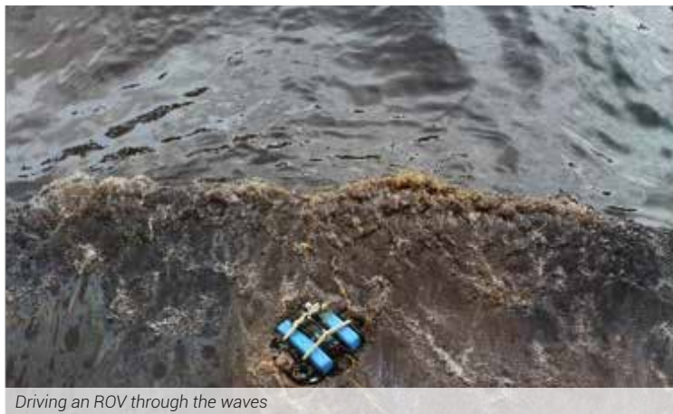
Oil spill tracking with an ROV at the Ohmsett tank in New Jersey
